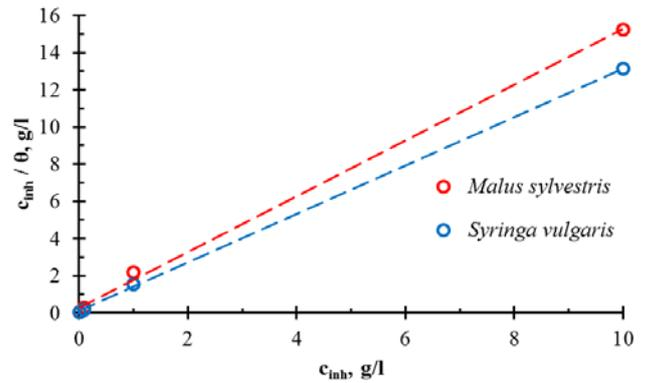
**Figure 4:** The plots of  $c_{inh}/\theta$  vs.  $c_{inh}$  for the adsorption of the *Malus sylvestris* flower extract and the *Syringa vulgaris* flower extract on the steel surface.
