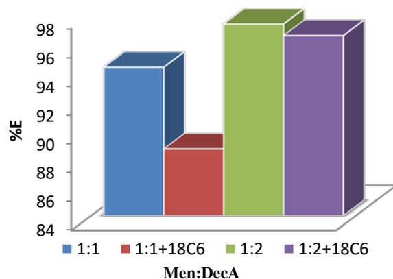
**Figure 4.** Comparison of Pb(II) ion extraction efficiency using Men:DecA solvent, with and without macrocyclic ligand 18C6 (SP contains:  $[\text{Pb}^{2+}] = 1 \cdot 10^{-4}$  mol/L and  $[\text{Pic}^-] = 4 \cdot 10^{-3}$  mol/L; pH=5; mixing time: 2h; used  $V(\text{HDES}) = 5$  mL,  $V(\text{SP}) = 5$  mL)
