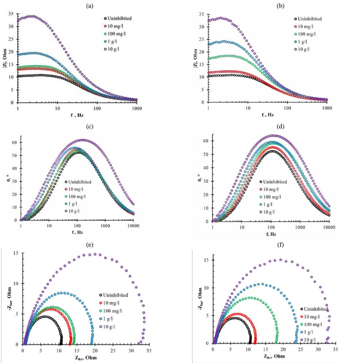
**Figure 3:** The Bode plots of steel in  $0.5$  M  $H_2SO_4$  with the different additions of (a), (c) the *Malus sylvestris* flower extract, (b), (d) the *Syringa vulgaris* flower extract, and the Nyquist plots of steel in  $0.5$  M  $H_2SO_4$  with the different additions of (e) the *Malus sylvestris* flower extract, (f) the *Syringa vulgaris* flower extract after 30 min of exposure.
