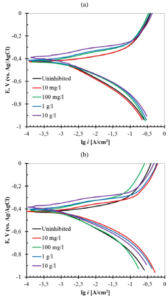
**Figure 2:** The polarisation curves of steel in 0.5 M H<sub>2</sub>SO<sub>4</sub> with the different additions of (a) the *Malus sylvestris* flower extract, (b) the *Syringa vulgaris* flower extract after 30 min of exposure.
